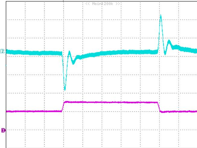
**Figure 6:** Output voltage response to step-change in load current (50%-75%-50% of  $I_{o, max}$ ;  $di/dt = 0.1A/\mu s$ ;  $V_{in}$  is 24V). Load cap: 10 $\mu F$  tantalum capacitor and 1 $\mu F$  ceramic capacitor. Top Trace:  $V_{out}$  (0.2V/div, 200us/div), Bottom Trace:  $I_{out}$  (5A/div). Scope measurement should be made using a BNC cable (length shorter than 20 inches). Position the load between 51 mm to 76 mm (2 inches to 3 inches) from the module
