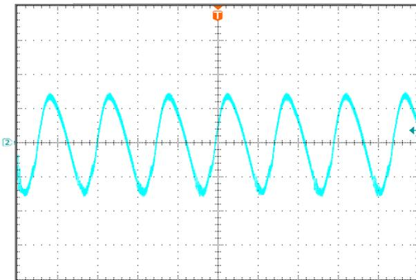
**Figure 12:** Output voltage ripple at nominal input voltage ( $V_{in}=48V$ ) and rated load current ( $I_o=10A$ ) ( $20mV/div$ ,  $2 \mu s/div$ ). Load capacitance:  $1 \mu F$  ceramic capacitor and  $10 \mu F$  tantalum capacitor. Bandwidth:  $20 MHz$ . Scope measurements should be made using a BNC cable (length shorter than 20 inches). Position the load between 51 mm to 76 mm (2 inches to 3 inches) from the module
