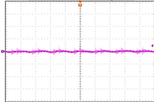
**Figure 10:** Input reflected ripple current,  $i_s$ , through a  $12 \mu H$  source inductor at nominal input voltage ( $V_{in}=48V$ ) and rated load current ( $5mA/div$ ,  $2 \mu s/div$ )
