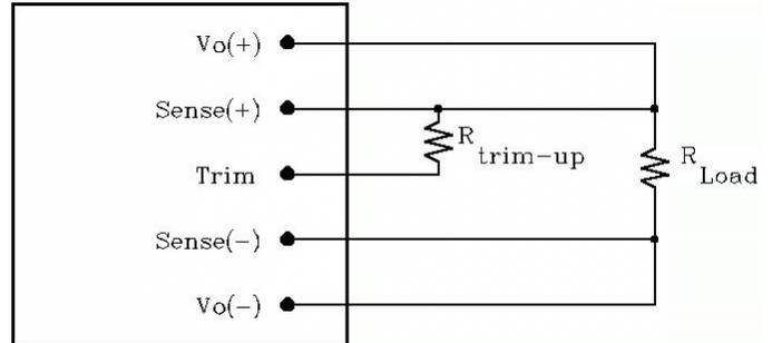
**Figure 17:** Circuit configuration for trim-up (increase output voltage)
