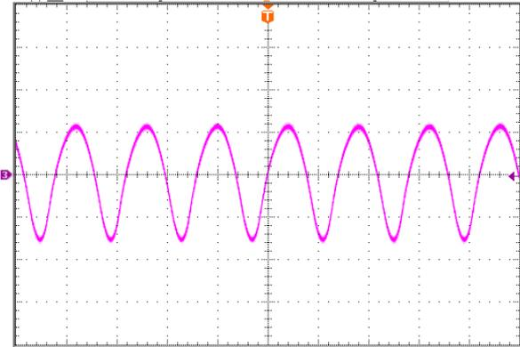
**Figure 9:** Input Terminal Ripple Current,  $i_c$ , at full rated output current and nominal input voltage ( $V_{in}=48V$ ) with  $12 \mu H$  source impedance and  $33 \mu F$  electrolytic capacitor ( $250mA/div$ ,  $2 \mu s/div$ )
