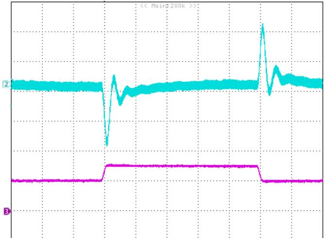
**Figure 7:** Output voltage response to step-change in load current (50%-75%-50% of  $I_{o, max}$ ;  $di/dt = 0.1A/\mu s$ ;  $V_{in}$  is 48V). Load cap: 10 $\mu F$  tantalum capacitor and 1 $\mu F$  ceramic capacitor. Top Trace:  $V_{out}$  (0.2V/div, 200us/div), Bottom Trace:  $I_{out}$  (5A/div). Scope measurement should be made using a BNC cable (length shorter than 20 inches). Position the load between 51 mm to 76 mm (2 inches to 3 inches) from the module
