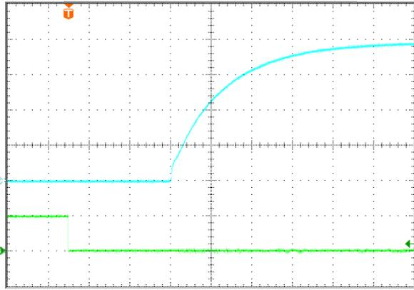
**Figure 4:** Turn-on transient at full rated load current (resistive load) (10 ms/div).  $V_{in}=48V$ . Top Trace:  $V_{out}$ , 3.0V/div; Bottom Trace: ON/OFF input, 5V/div
