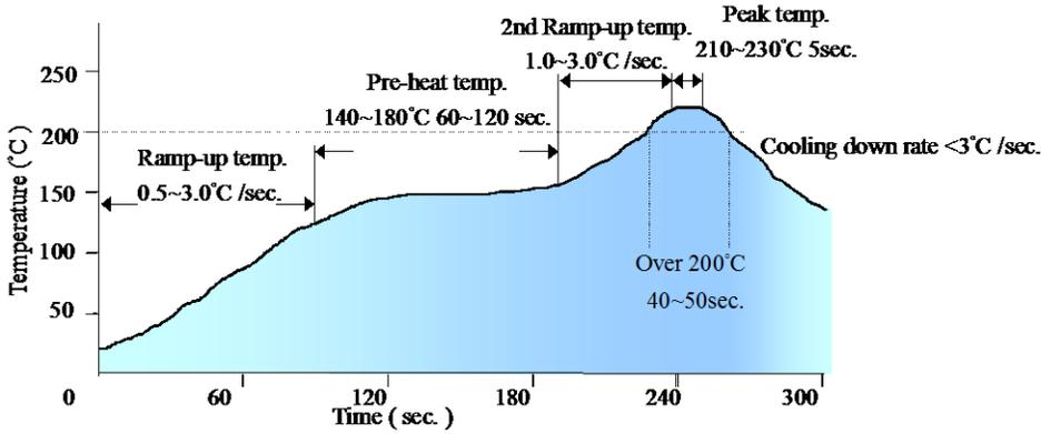
Note: The temperature refers to the pin of E36SC, measured on the +Vout pin joint.
