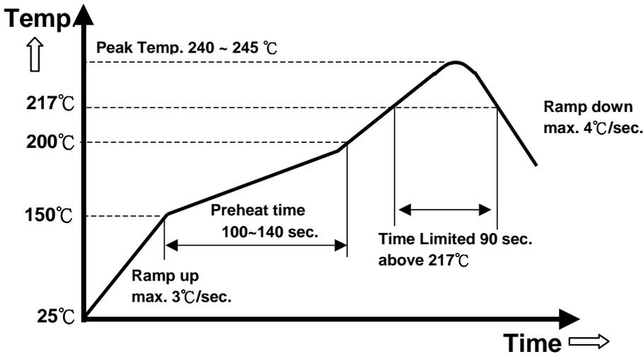
Note: The temperature refers to the pin of E36SC, measured on the +Vout pin joint.
